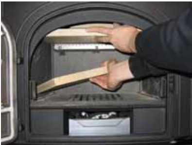
c. Remove the firebrick from the back-wall
