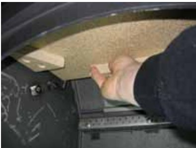
e. The upper baffleplate is removed from the brackets and lifted out of the fire-chamber
