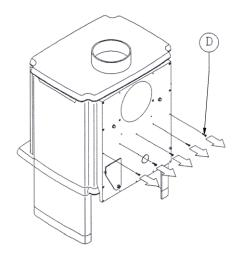
2.2 The 5 screws shown on the drawing as (D) are unscrewed and kept. These are to be re-used when fitting the air box.
