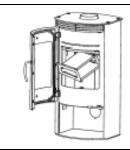
4. Place the baffle plate into the stove as shown above. The safety lock section should be on top and face out toward front of the stove.
