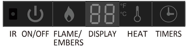
**a.IR:** Receiving infra-red signals(inputs)
